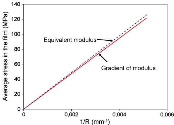
Fig. 9. Relationship between average stress in the film and curvature of the sample obtained by FEM for an average uniform modulus or a gradient of modulus.
