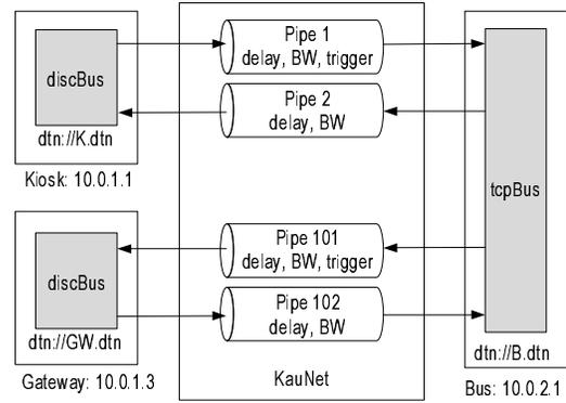
Figure 7: KauNet Setup for the Village Example.
