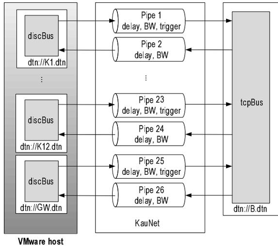
Figure 11: KauNet Setup for the Multiple Kiosk Example.
