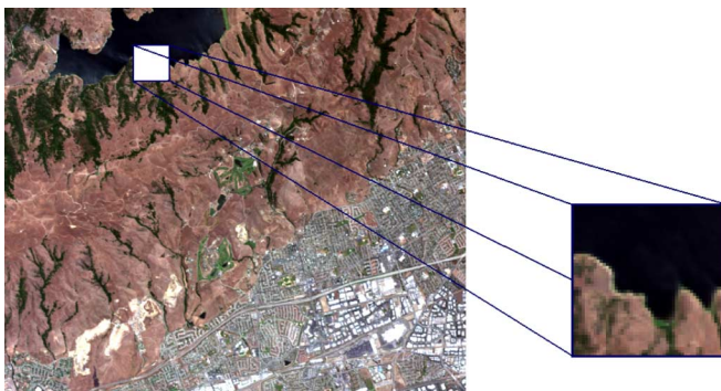
Fig. 6. Real hyperspectral data: Moffett field acquired by AVIRIS in 1997 (left) and the region of interest shown in true colors (right).
