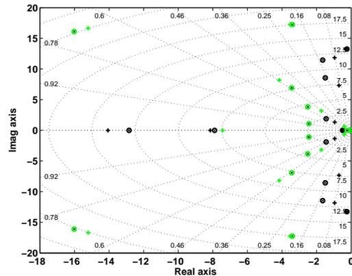
Fig. 5. Eigenvalue selection to solve equation (4): open-loop poles of  $P_o$  are marked with black  $+$ ; open loop poles of  $K_r$  are marked with green  $+$ ; 24 closed-loop poles are marked with  $o$ : the green ones are affected to state-estimation dynamics ( $\text{spec}(A_o - K_f C_o)$ ) and the black ones are affected to state feedback dynamics ( $\text{spec}(A_o - B_o K_c)$ ).
