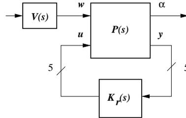
Fig. 2. Interconnection structure of the plant  $P$  and initial controller  $K_r$ .
