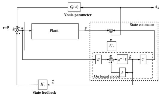
Fig. 1. Observer-based realization of a given controller using YOULA parameterization.
