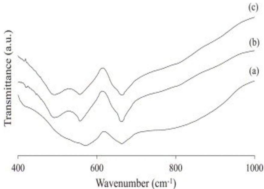
From XRD and FTIR analyses, it is concluded that during the calcination of a mixture of cobalt and aluminium chlorides, the formation of  $\text{CoAl}_2\text{O}_4$  begins to occur above  $800\text{ }^\circ\text{C}$  and is not finished at  $1200\text{ }^\circ\text{C}$ . Moreover, the determination of the molar ratio Al/Co by X-EDS reveals great heterogeneities of the chemical composition, that ratio varying in the range 1.1–4.3 according to the investigated area.
