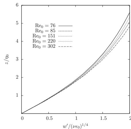
FIG. 4. Profiles of the rms normal velocity fluctuation scaled by the Kolmogorov scales at the surface ( $\nu, \epsilon_0$ ).
