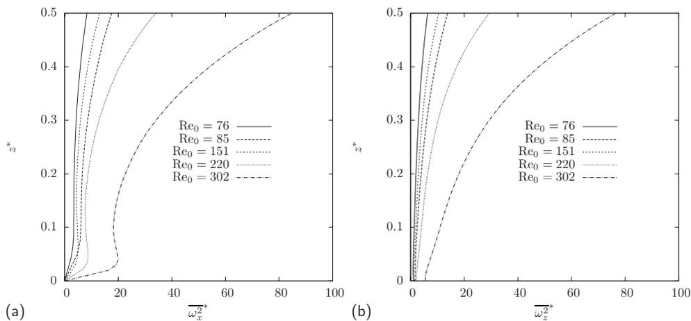
FIG. 6. Profiles of the vorticity variances above the surface. (a)  $\overline{\omega_x^2}$  and (b)  $\overline{\omega_z^2}$  [all quantities normalized by the turbulent scales at the surface ( $k_0, \epsilon_0$ )].
