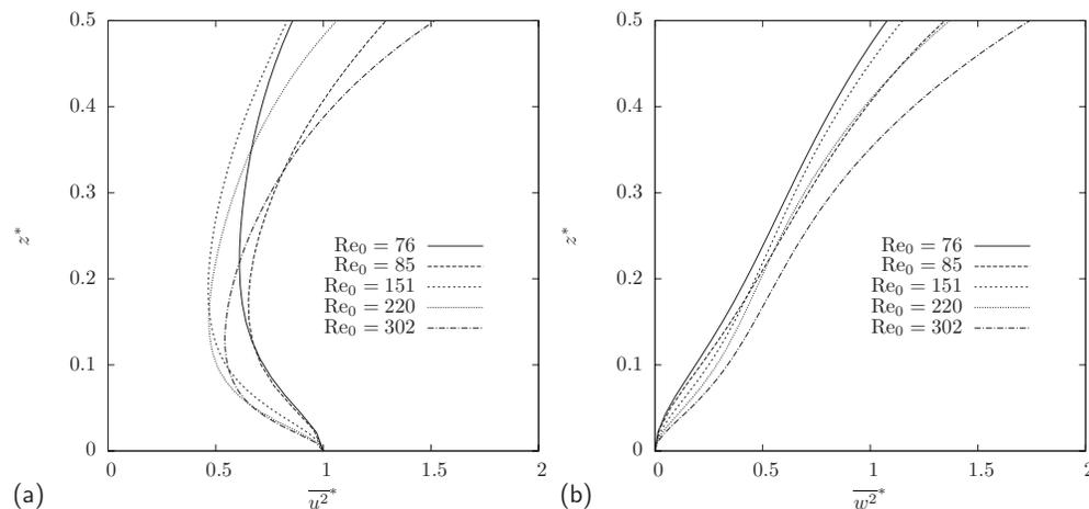
FIG. 2. Profiles of the Reynolds stresses above the surface. (a)  $\overline{u^2}$  and (b)  $\overline{w^2}$  [all quantities normalized by the turbulent scales at the surface ( $k_0, \epsilon_0$ )].
