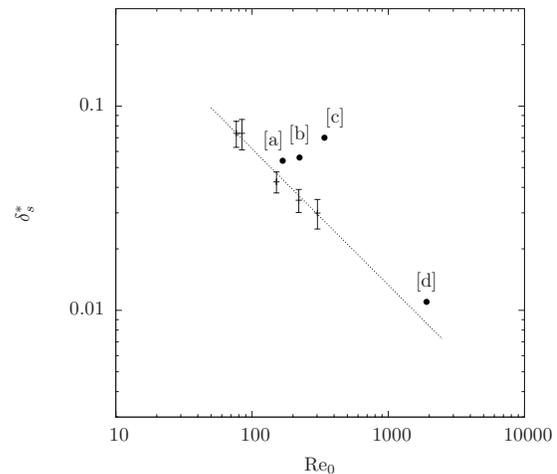
FIG. 8. Reynolds-number dependence of the slip-layer thickness. Error bars, present data; dashed line, Eq. (11); solid dots, literature data with [a] Ref. 4, [b] Ref. 6, [c] Ref. 11, and [d] Ref. 13.
