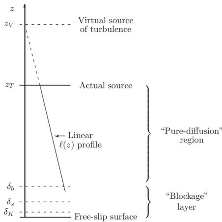
FIG. 1. Theoretical sketch of the interaction between a plane source of turbulence and a free-slip surface. The source and the surface are contained in parallel  $(x, y)$  planes.
