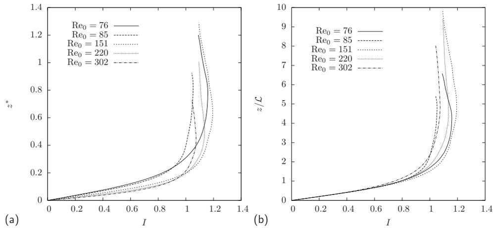
FIG. 3. Profiles of the isotropy parameter outside the turbulent-production region. (a)  $z$  is normalized by the turbulent scales at the surface ( $k_0^{3/2}/\epsilon_0$ ) and (b)  $z$  is normalized by the slope of the profile at the surface.
