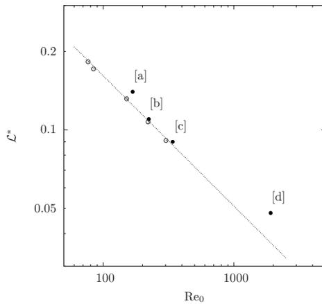
FIG. 5. Reynolds-number dependence of the outer layer thickness:  $\mathcal{L}^*$  is plotted against the value of the turbulent Reynolds number at the surface. Open symbols, present data; dashed line, Eq. (9) with  $A=0.62$ ; filled symbols, literature data with [a], Ref. 4, [b] Ref. 6, [c] Ref. 11, and [d] Ref. 13.
