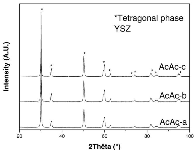
Fig. 4. Water influence study: diffraction patterns of powders (AcAc synthesis).
