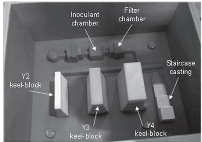
Fig. 2. Pattern used for preparing the poured castings.
