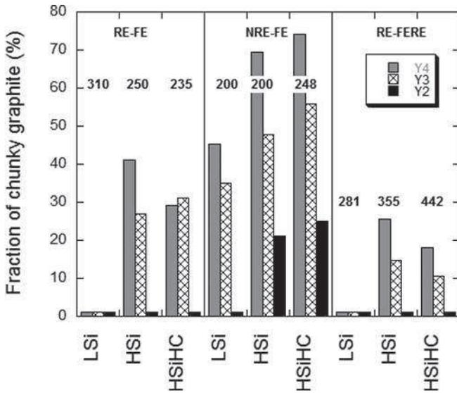
Fig. 5. Effect of silicon and carbon contents on chunky graphite amount. Numbers are nodule counts (mm<sup>-2</sup>) measured at the bottom of Y2 blocks.
