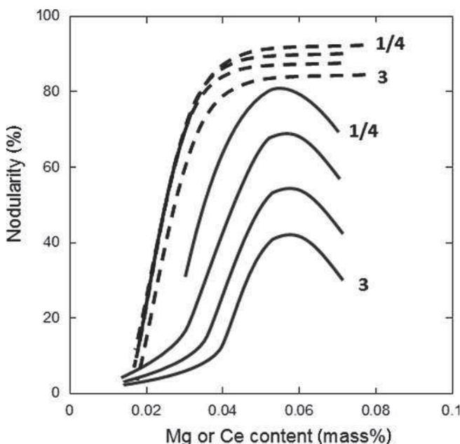
Fig. 1. Effect of magnesium (dashed lines) and cerium (solid lines) on nodularity for various section sizes,  $1/4$ ,  $1/2$ , 1 and 3 inches. After White et al. [1].
