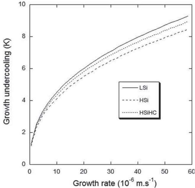
Figure A1. Evolution of the dendrite tip growth undercooling with the growth rate for Fe–C–Si alloys with compositions corresponding to LSi, HSi and HSiHC alloys.
