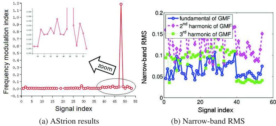
**Figure 10: Diagnosis of the anonymous wind turbine gearbox: (a) frequency modulation index obtained in AStrion by demodulating the side-band series around the second harmonic of GMF modulated by shaft speed, and (b) narrow-band RMS computed with a bandwidth of 3 side-bands on both sides of the carrier frequency.**
