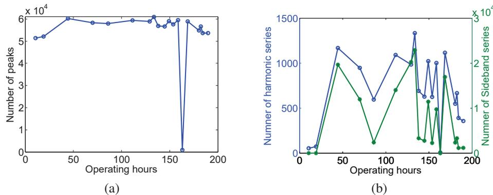
**Figure 3: Results of the detection of peaks, harmonic series and side-band series on the 19 signals of accelerometer (+y), mounted on the main bearing of the test rig from 10.62 to 189.85 operating hours: (a) number of peaks detected, and (b) number of harmonic and side-band series detected.**
