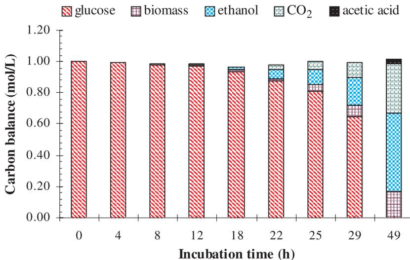
mine the carbon in the liquid substrate and products. The gas analysis of the fermentor outlet gave, after integration, the carbon atoms in the carbon dioxide produced. For the fermentation at 25 °C, global and instantaneous carbon balances were made. Figure 4 shows the evolution in the carbon balance between glucose and the different by-products of the fermentation.
