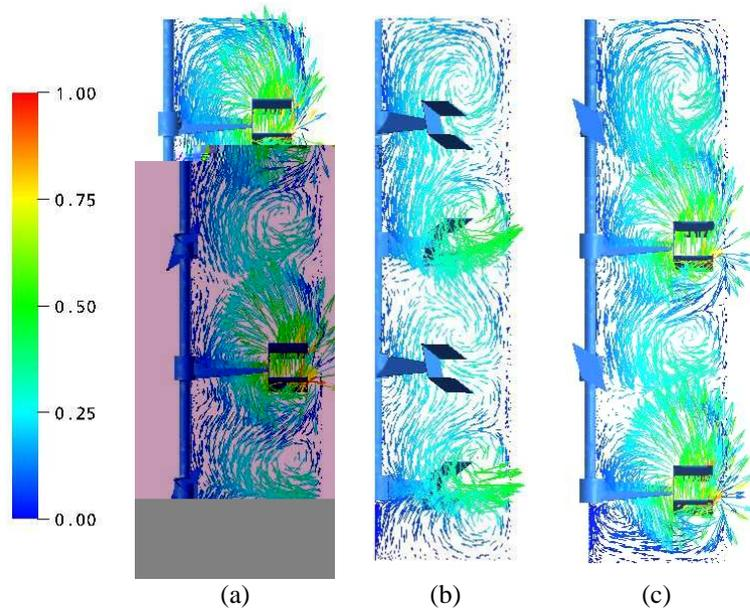
**Figure 2:** Radial-axial flow patterns for IMIG-90 at  $Re = 60$ . (a)-(c) planes varying in the azimuthal direction. Vectors coloured by the velocity normalized by the impeller tip speed ( $1.75 \text{ ms}^{-1}$ ).
