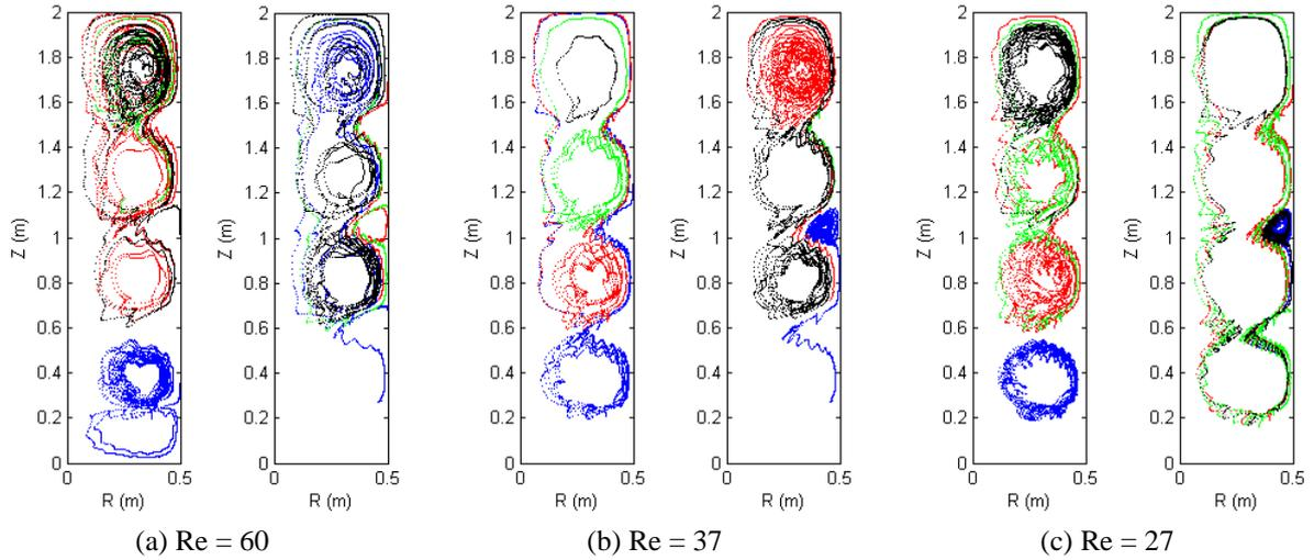
**Figure 5:** 3-dimensional particle tracking projected on to a radial-axial plane for IMIG-45CW. (a) Re = 60, (b) Re = 37, (c) Re = 27. Particle are released in level with the 4 Intermigs (■  $z = 0.27$  m; ■  $z = 0.72$  m; ■  $z = 1.17$  m, ■  $z = 1.62$  m) and at two radial positions  $r = 0.25$  m (left figure) and  $r = 0.45$  m (right figure).
