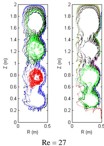
**Figure 7:** 3-dimensional particle tracking projected on to a radial-axial plane for IMIG-45ACW-C at  $Re = 27$ . Particle are released in level with the 4 Intermigs (■  $z = 0.27 \text{ m}$ ; ■  $z = 0.72 \text{ m}$ ; ■  $z = 1.17 \text{ m}$ , ■  $z = 1.62 \text{ m}$ ) and at two radial positions  $r = 0.25 \text{ m}$  (left figure) and  $r = 0.45 \text{ m}$  (right figure).
