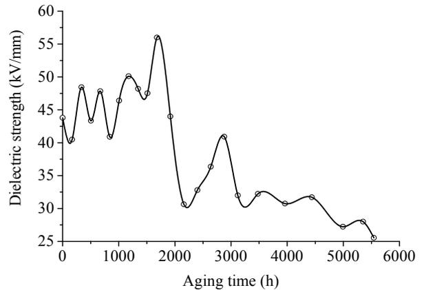
Fig. 6. Dielectric strength changes versus aging time.
