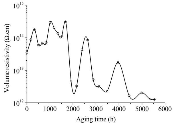
Fig. 5. Volume resistivity evolution versus aging time.
